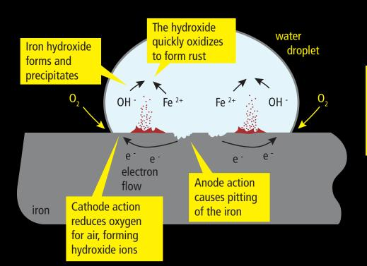
Electrochemical cell action driven by the energy of oxydation continues the corrosion process
